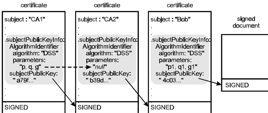
Figure 8 - Parameter Inheritance in Certification Path
