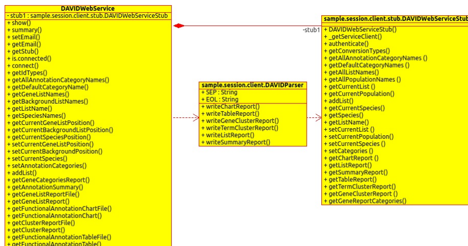
Figure 1: R-to-Java class diagram. RDAVIDWebService uses rJava to access/control DAVID web service through RDAVIDWebServiceStub and parse the reports back to R by DAVIDParser . Note that operation signatures have been omitted for simplicity.
